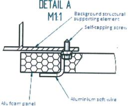
Aluinvent Designium® cladding system – Load bearing capacity of fastening systems
